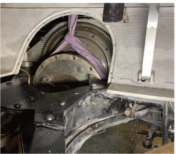
Whilst on the subject of AYF the car has completed 24 miles and even though this run was short it has shown a noisy bearing in the gearbox which is now replaced with a NOS original Hoffman 140. With the gearbox out of the chassis, I have taken advantage of the improved access to remove the clutch as it was suffering from a violent juddering when starting from rest - cause as yet unknown but I'm on its case.
